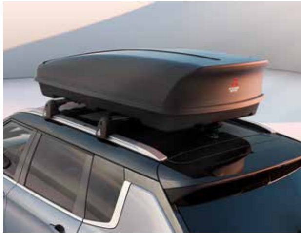
▼ Rigid roof box Capacity; 380, 480 or 630 liter. For partnumbers see QRL
