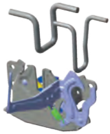
Hood safety mechanism with double striker
